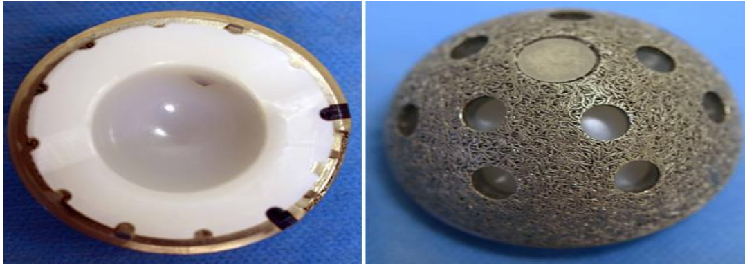
(Left) The acetabular component shows the plastic (polyethylene) liner inside the metal shell. (Right) The porous surface of this acetabular component allows for bone ingrowth. The holes around the cup are used if screws are needed to hold the cup in place.
